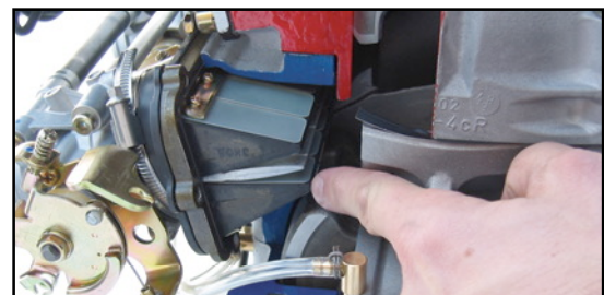
Reed valves used in Fusion 900 engine.
