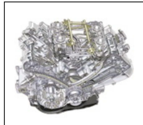
90 degree V-4 engine found in Honda VFR 800 motorcycle.
