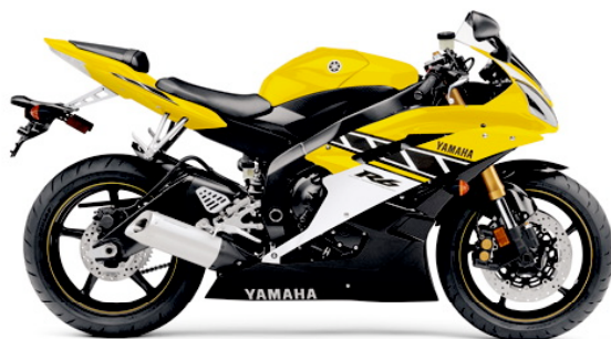
The engine in the 2006 R6 has a 17,500 rpm redline!
