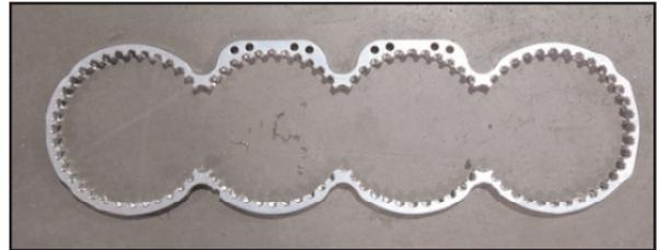
*The aluminum reinforcement (above) that will be used to strengthen the engine block, in position (below).*
