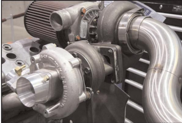
*The two turbochargers (set sequentially) that will be used to provide the necessary boost.*
