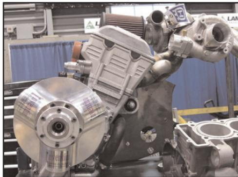
*The Hydradjust (by Inventium) clutch is one of the components being tested. Managing 500 HP is a tall order, however.*
