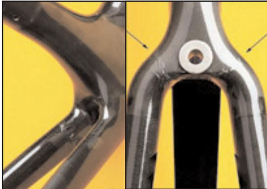
Fractures in this bicycle frame illustrate how challenging it can be to identify delamination in CFRP's.
