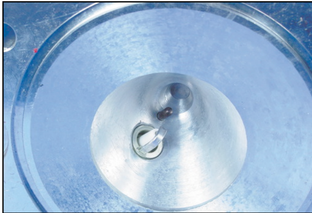
Injector position in the combustion chamber. Please note that the spark plug gap is indexed in the direction of the injector nozzle (to ensure a more efficient combustion in stratified mode.)
