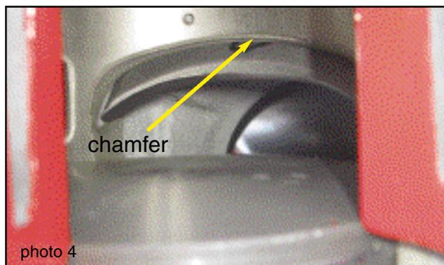
edges – an important step. Production parts are usually OK in this respect, but cylinders freshly bored or coated may need port edges smoothed with an abrasive-charged rubber wheel.
