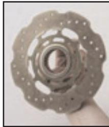
The ventilated disc (left) used on the new Yamaha FX Nytro, and the "wave" rotor as found on the Ski-Doo REV-XP sleds.
