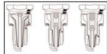
«Hot» plug (left) with substantial exposed insulator. At the extreme right a «cold» plug with much less exposed insulator
